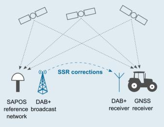
To access the corrections, a DAB+ receiver module with the necessary demodulator software is integrated in the Alberding A10-RTK GNSS rover receiver.
